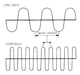
Every radio station in the world is assigned one or more specific frequencies (or wavelengths) on which it may transmit its signals. The radio RECEIVER selects the frequency (or wavelength) and reproduces the broadcast.
